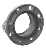
Style 994 HDPE flange adapter for HDPE pipe permits direct connection of ANSI Class 125 and 150 flanged components into HDPE systems. No fused adapters are required. The housing bolts onto the pipe end with sharp teeth to grip the pipe with tongue-and-groove for positive axial alignment. The Style 994 gasket seals on the pipe O.D. and directly to the flange face. No standard flange gasket is required.
