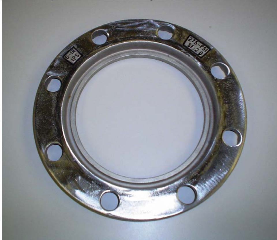
Figure 4 Cast Stainless Steel, Lap-Joint Flange, 6-inch IPS
