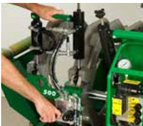
**AVAILABLE HYDRAULIC CLAMPING** Save time and increase productivity by eliminating manual-crank clamp knobs on 618 machines. **To purchase, add "HC" to the end of the part number above.**
