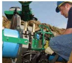
**REMOVABLE CARRIAGE** The TracStar carriage can be easily removed for tight installations. The outer fixed jaw and skid can also be removed converting it to a 3-jaw machine for an even more compact unit.
