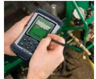
**DATALOGGER® COMPATIBLE** Record heat-er temperature and fusion pressure profiles over time in adherence to supported fusion standards. **See pg 48 for more information.**
