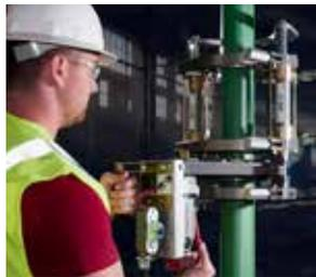
**FLEXIBLE TO MEET THE JOB DEMANDS** Thanks to the Acrobat's narrow jaw construction and compact package, flange-to-pipe, fitting-to-pipe and even fitting-to-fitting fusions can be done with ease.
