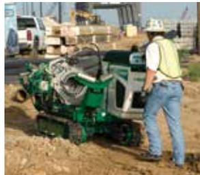
**SELF-PROPELLED** TracStar machines are mounted on all terrain rubber tracks and easily maneuverable on any jobsite with independent controls for each track.
