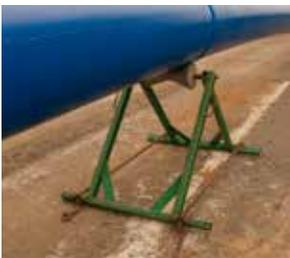
**SAVE WEAR AND TEAR ON EQUIPMENT** McElroy pipe stands are adjustable for uneven terrain so that pipe is supported at the same height as the fusion machine.
