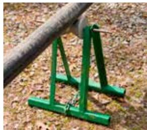
**INCREASE PRODUCTIVITY** Instead of moving the machine for each joint, pipe stands allow the fused pipe to be pulled through the machine while rolling a new stick in to place.
