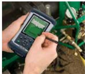
**DATALOGGER® COMPATIBLE** Record heat-er temperature and fusion pressure profiles over time in adherence to supported fusion standards. **See pg 48 for more information.**
