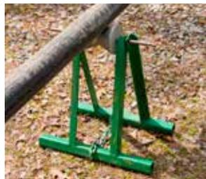
**INCREASE PRODUCTIVITY** Instead of moving the machine for each joint, pipe stands allow the fused pipe to be pulled through the machine while rolling a new stick in to place.
